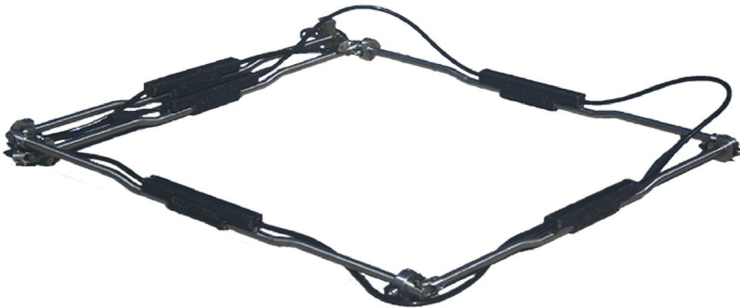
Figure 1: GEOSTRING segment folded for transport
