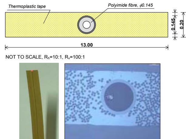
Figure 4: Cross-section picture and micrograph of the sensing tape: SMARTape
