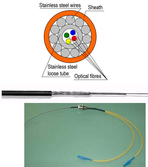
Figure 3: Extreme temperature sensing cable design and termination
