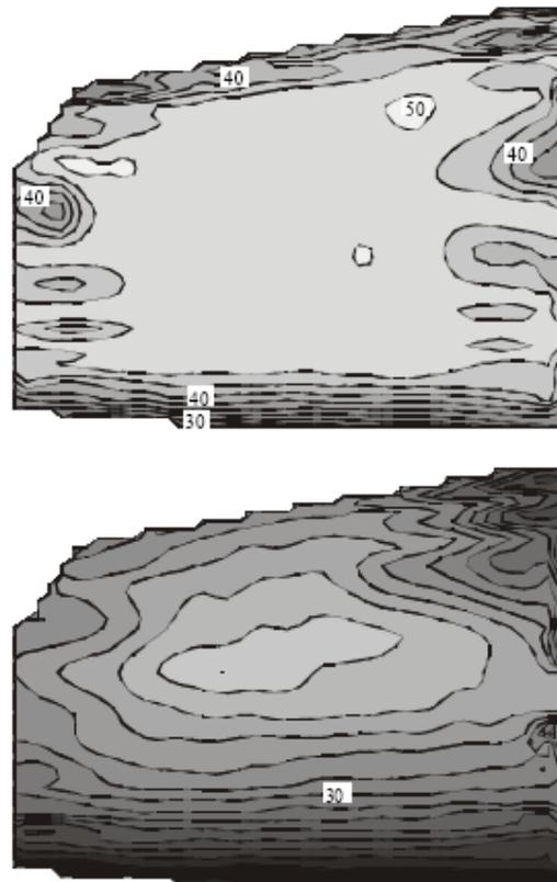
Figure 6: Luzzone Dam raising works and temperature measurements in the Luzzone Dam 15 and 55 days after concrete pouring (courtesy of L. Thévenaz)
