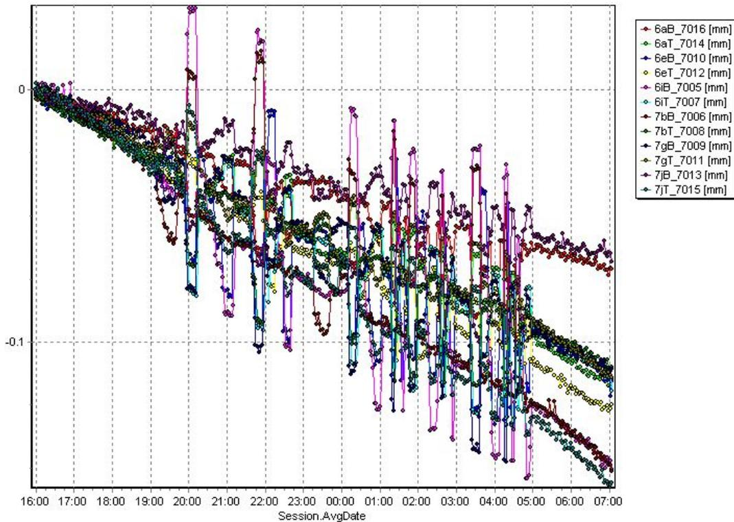
Figure 6: Raw data acquired on the SOFO strain sensors during the test.
