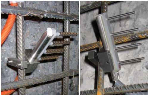
Concrete corrosion and Humidity sensors
