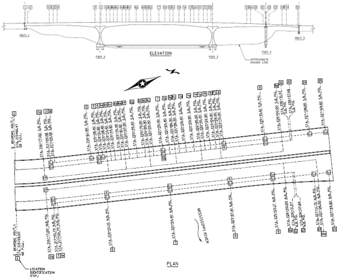
Figure 2: Global overview of the I-35W Bridge health monitoring system (courtesy of Flatiron Mason)
