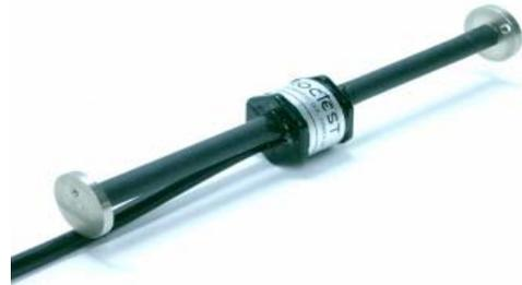
Vibrating Wire Strain Gauge
