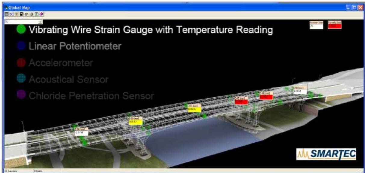
Figure 4: SDB View Software interface (simulation)
