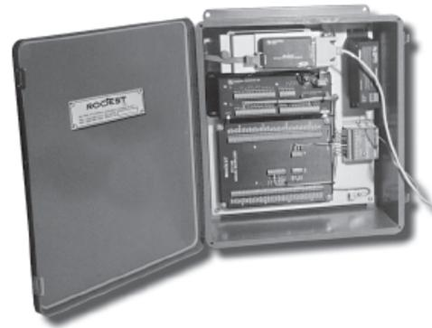
Vibrating wire and temperature sensors datalogger
