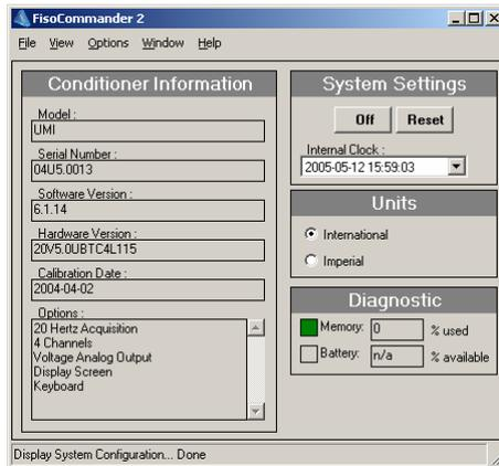
2. In the **Units** box, select the radio button corresponding to the desired measurement units.
