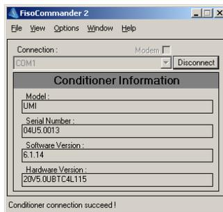
The **Connection** drop-down list provides the list of port options that are available on your PC to establish a connection with a UMI unit.
