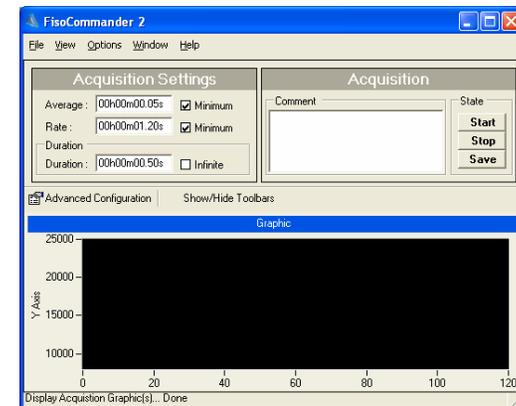
It is possible, from this window, to start and stop real-time acquisitions. You may also determine the averaging time, the rate, as well as the duration of the acquisition. Data obtained through this acquisition mode can be saved to a file at the end of the session.
