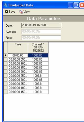
From the **Downloaded Data** window, you will obtain the date of the acquisition, and the average and rate parameters that were defined for the selected acquisition session. The table underneath the data parameters lists all the data points, along with the time each point was taken, the first data point starting at zero.
