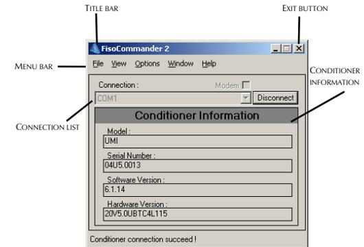
Figure 3. FISOC Commander 2 connection window
