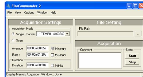
2. Select the radio button of the desired scanning mode for your acquisition: **Single Channel** or **Scan**.
