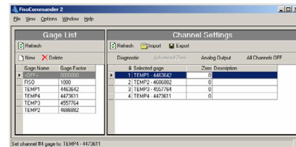
3. Click on the channel you want to use. Make sure that your pointer is located on the **Channel N°** column. The channel will be displayed in bold.
