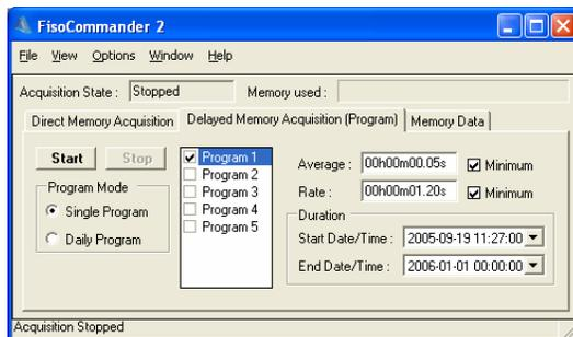
Up to five programs may be stored in the unit and executed through the FISOCommander software. The data obtained through a delayed memory acquisition is stored in the unit's internal memory and will have to be downloaded before being able to store it to a computer.
