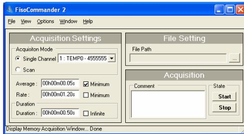
In the **Acquisition Settings** group, you define the acquisition mode, as defined previously, as well as all the necessary parameters to determine the duration and the frequency of each reading.
