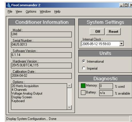
The **System Settings** group provides controls to turn the unit off, to reset the conditioner's information to factory default values, to adjust the internal clock, and to select the measurement units that will be used for the acquisitions. It also provides a quick diagnostic chart to evaluate the unit's performance.
