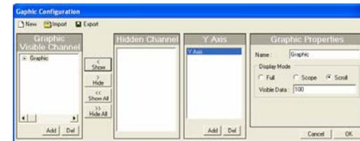
2. Make sure that the channels that will be used to plot the graph are present in the **Graphic Visible Channel** table.
