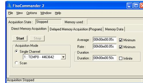
2. Configure the parameters (average, rate, and time) according to your test requirements.
