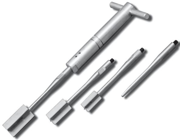
**PORTABLE HANDHELD VANE TESTER
