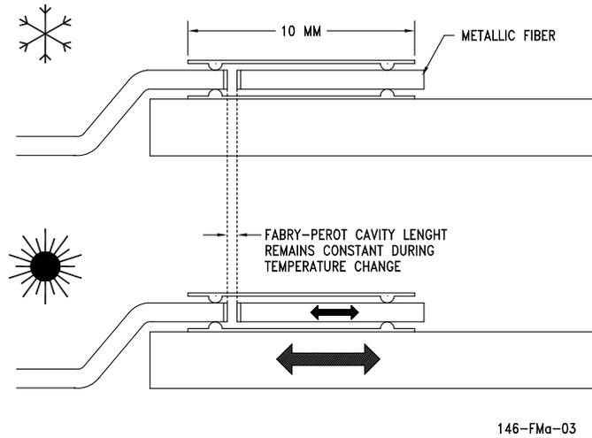
Figure 2: Principle of self-compensation mechanism
