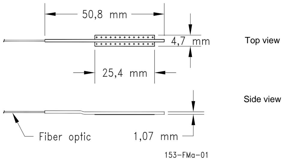
Figure 3: SFO-W Spot Weldable Strain Gauge
