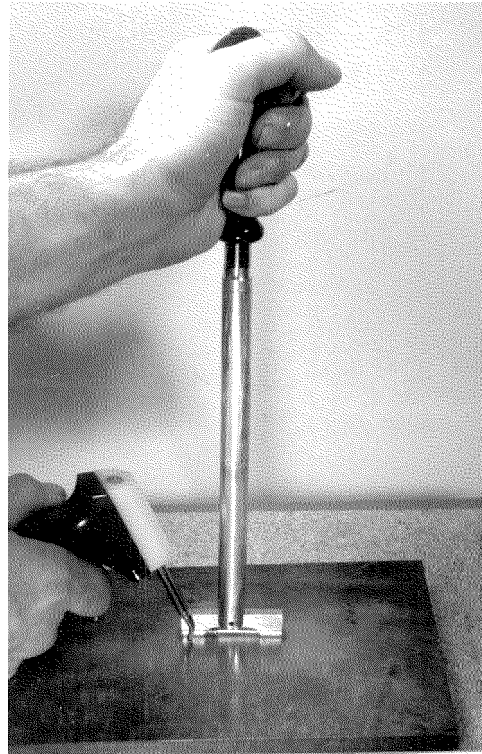
Figure 4 Photograph showing gauge installation
