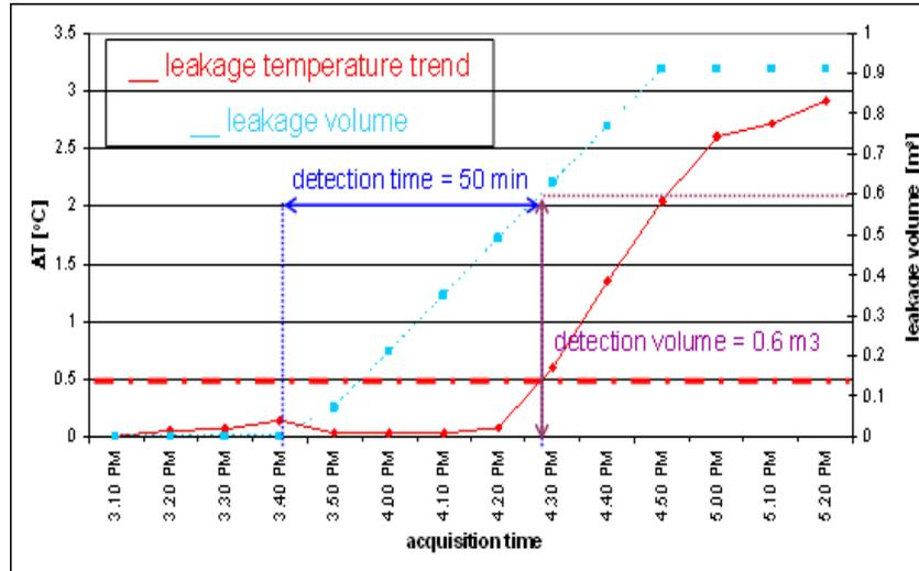
Fig.7. Temperature and leaked volume evolution at leak location 3.
