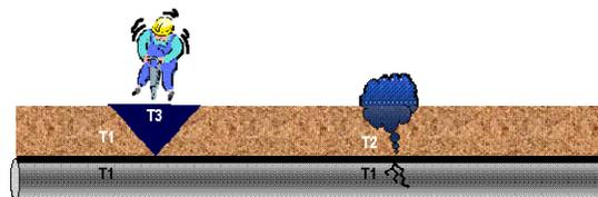
Fig.3. Detection of a gas leak through a cable placed above the pipeline.
