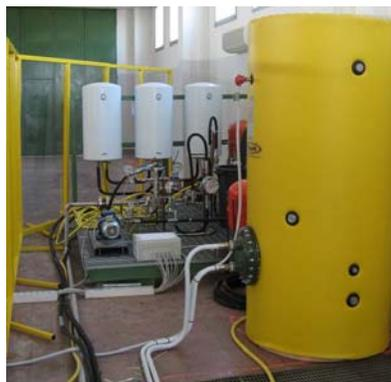
Fig. 12. Liquid leakage circuit.
