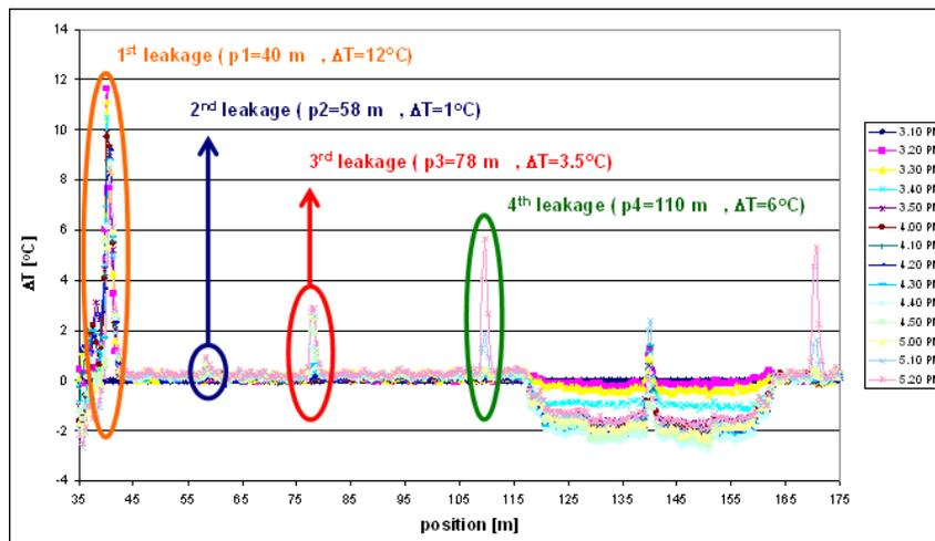
Fig.6. Relative temperature data for the leakage test.
