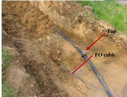
Fig.4. Leakage detection simulation arrangement. Several taps, with volume meters are used to generate controlled leaks.
