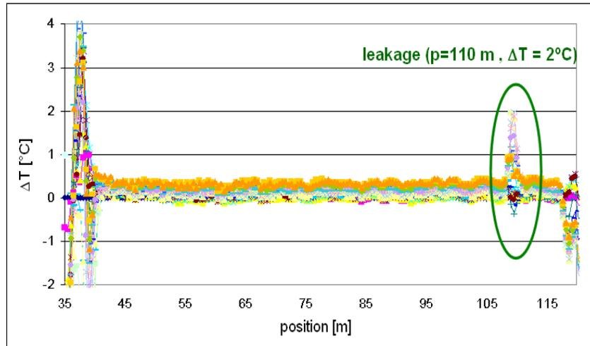
Fig.8. Relative temperature data for the leakage test.
