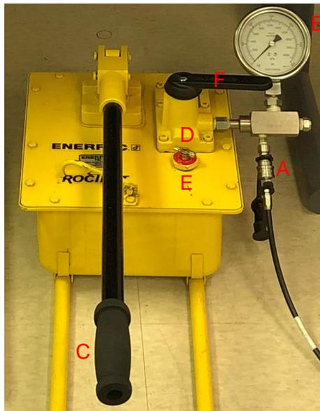
Standard Model Enerpac P462 Pump main specifications:
