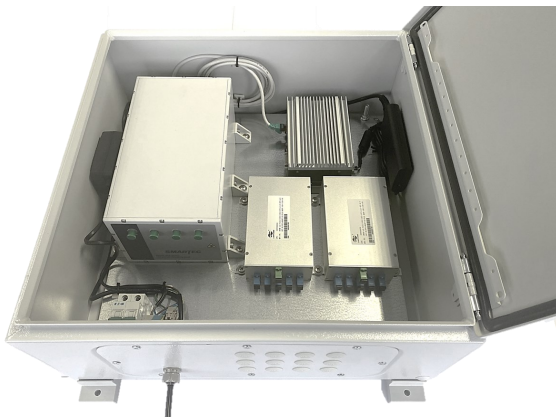
Outdoor enclosure including SOFO VII unit with two splitters and field PC.
