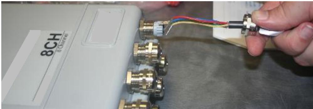
Figure 3-2: Sensor Valve Connection
