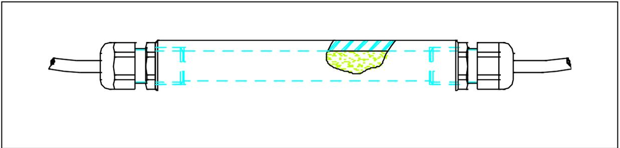
Figure 3: Cable splicing assembly with PVC connectors for IRC-41A cable (FR-1135050900)
