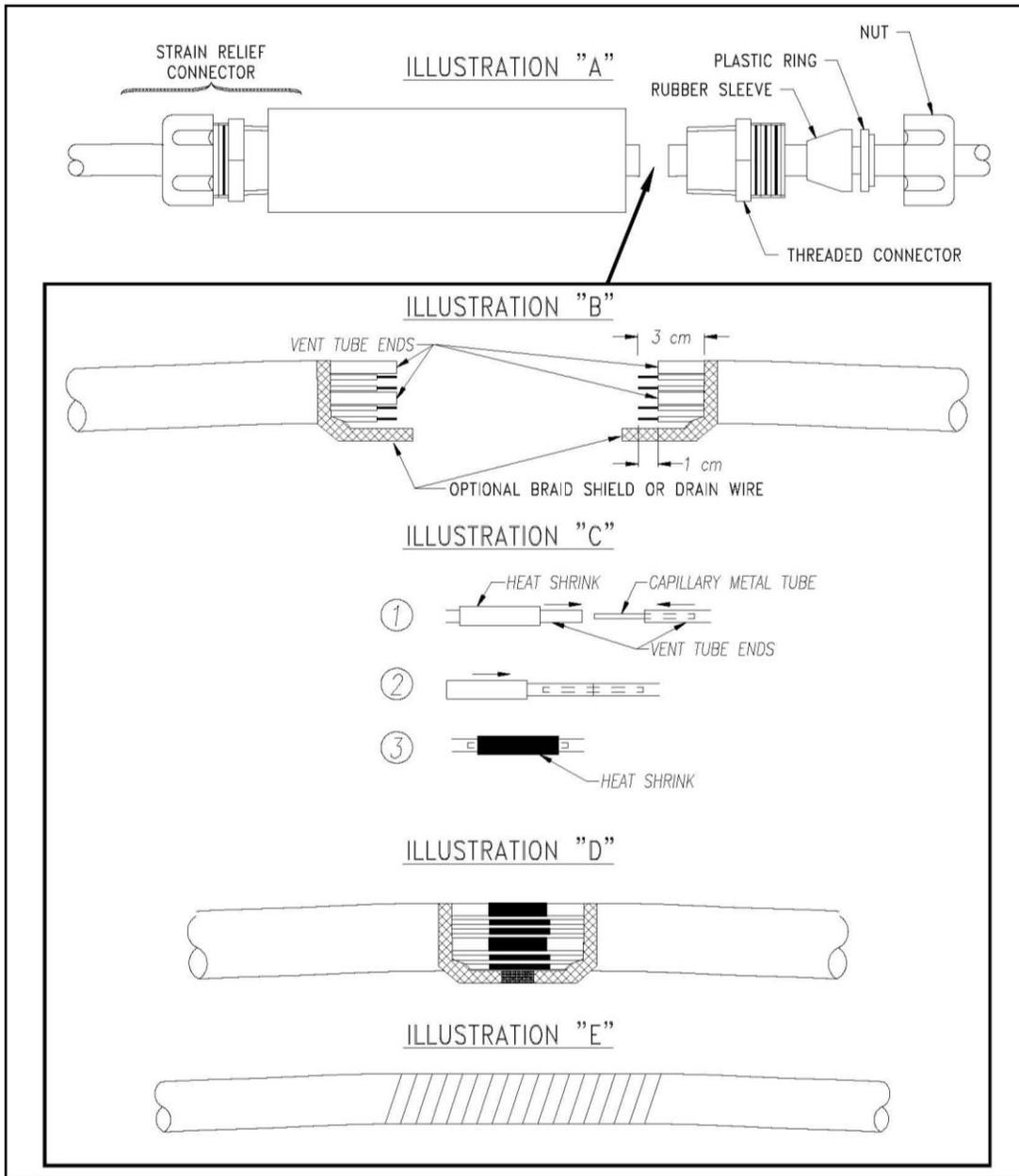
Figure 1: Steps for cable splicing with T&B connectors
