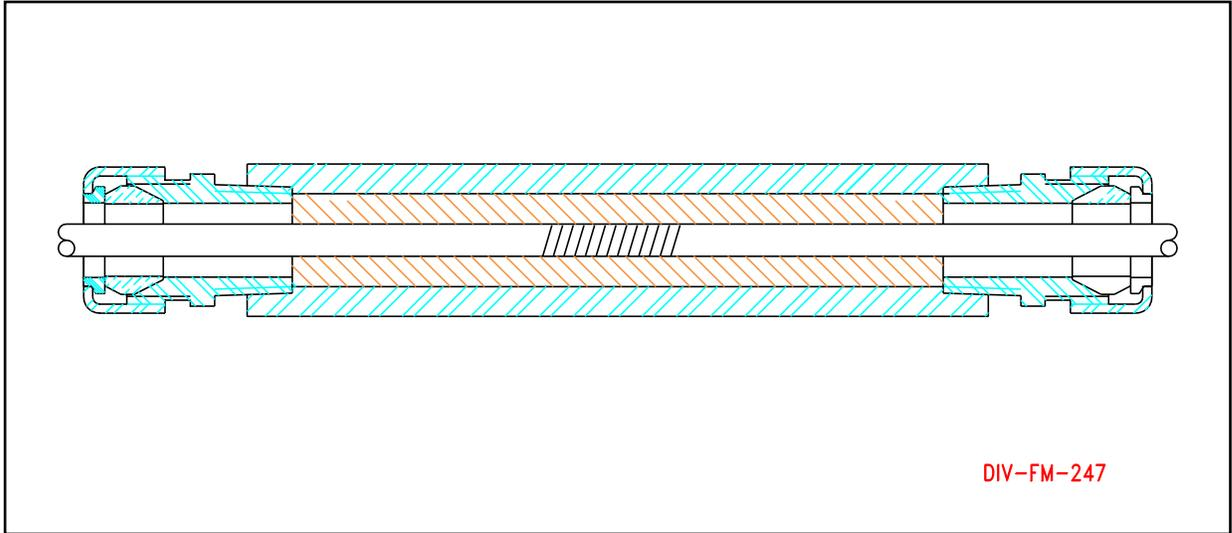
Figure 2: Cable splicing assembly with T&B (metal) connectors (FR-1135050900C)
