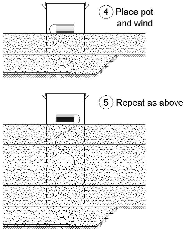
Figure 6: Procedure to route vertically cables
