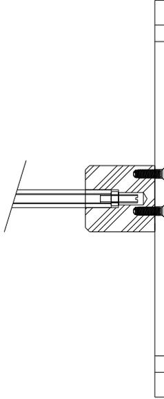
**Once the sensor assembled, take care not to rotate one flange relative to the other. Relative rotation of the end flanges could damage the spring and then the instrument.**
