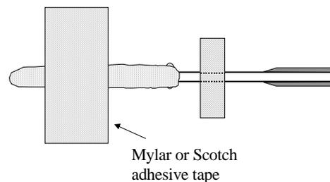
*Reminder: The key for successful strain gauge bonding is to have a good contact between the gauge and the specimen to measure.*
