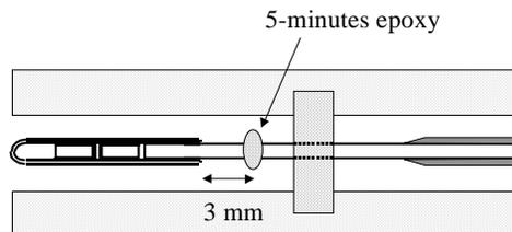
*Reminder: To avoid surface contamination, do not touch the micro-capillary of the Fiber-Optic Strain Gauge with your hands. The gauge micro-capillary must be free of grease, dust, etc. If necessary, use a Duster can or clean dry air to blow away dust, dirt and grit on the micro-capillary.*
