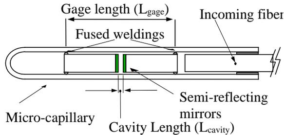
Relation between the length of the cavity ( $L_{cavity}$ ) and the strain ( $\varepsilon$ ) is determined by the following formula:
