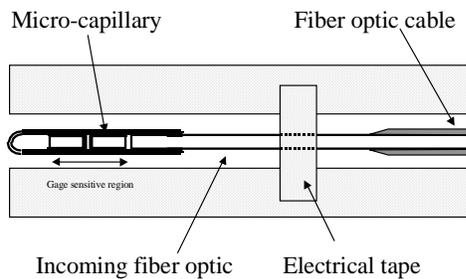
*Note: The gauge micro-capillary is made of glass and doesn't have any protective coating so it should be handled with care prior to bonding the gauge. Any scratches made to the glass micro-capillary may impair the efficiency and the lifetime of the gauge.*
