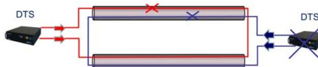
*Redundant setup with two interrogators and looped fibers.*
