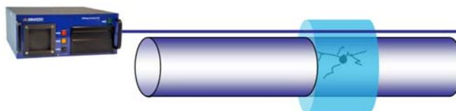
*In the event of gaseous leak, the temperature drops due to the gas expansion (Joules Thomson effect).*
