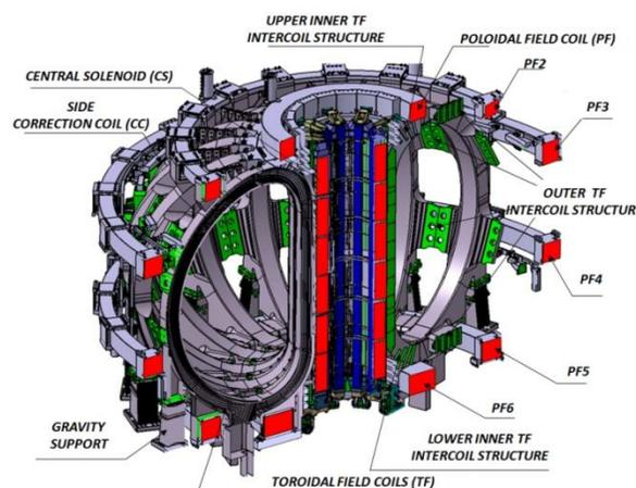
Fig. 1. Overview of the ITER superconducting magnet systems. The feeder lines are not shown.
