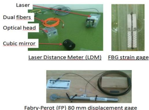
Fig. 5. A SMARTEC LDM long range (20 m) displacement gage (top left), a dual FBG strain gage assembled on a spot-weldable stainless steel sheet; it uses a temperature and radiation compensation FBG gage (top right). A large displacement FP displacement gage (bottom).
