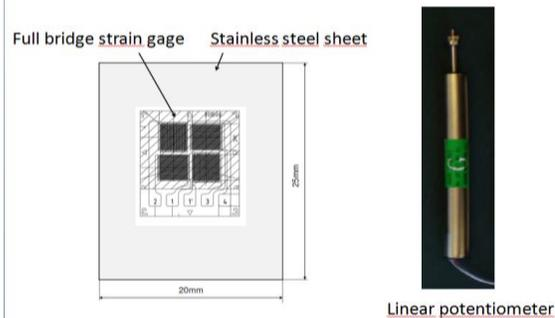
Fig. 3. An HBM full bridge 4 sensors strain gage pre-assembled on a spot-weldable stainless steel sheet (left), and a commercial linear displacement potentiometer adapted to ITER environment (right).
