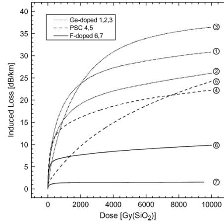
Fig. 2. Induced losses in irradiated (Co 60) commercial radiation-hard fibers as function of dose. Fluorine-doped fibers (curves 6,7) show practically no change in optical transmission.
