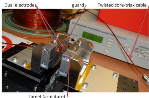
Fig. 4. Fogale-Nanotech bi-directional displacement capacitive sensor.
