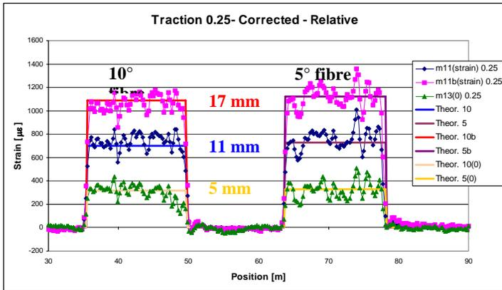
Figure 16. Results of the traction test and comparison with theoretical prediction
