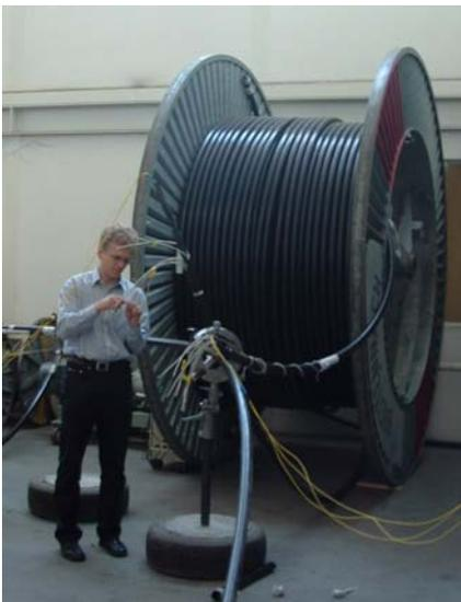
Figure 18. Liner heating test by electrical current injection
