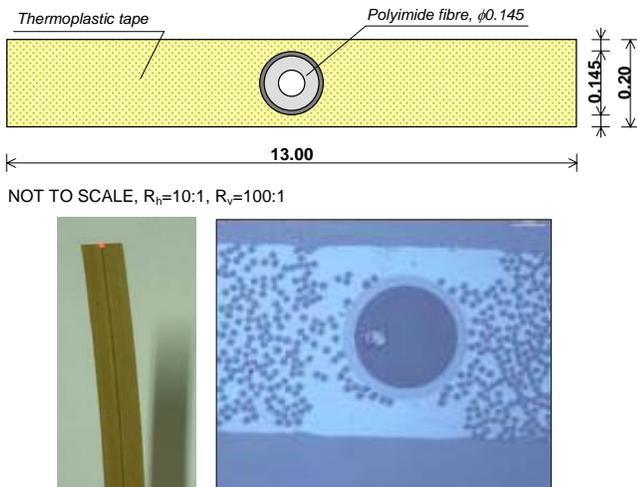
**Figure 4: Cross-section picture and micrograph of the sensing tape (SMARTape)**
