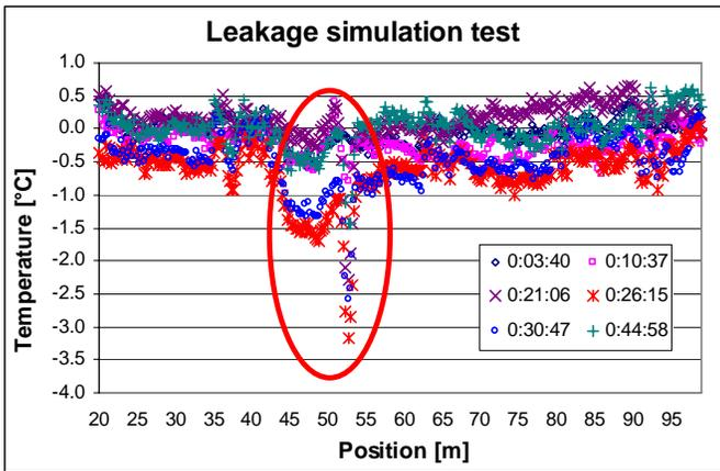
Figure 12. Results of leakage test; leakage is detected as temperature change
