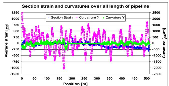
Figure 10. Cross-section strain and curvatures distribution measured by SMARTape sensors
