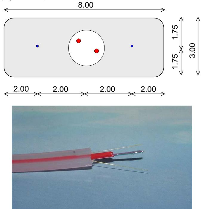
**Figure 5: SMARTprofile cross-section and sample. The red tube contains the free fibers**
