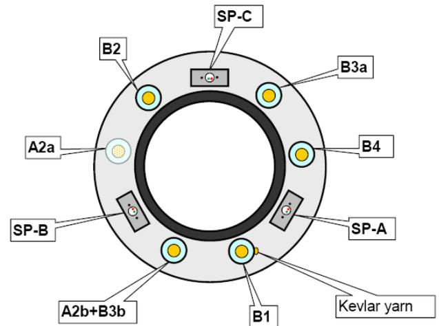
**Figure 15. PDT-Coil Cross-section. The fiber optics sensing SMARTprofiles are designated by SP-A, SP-B and SP-C.**
