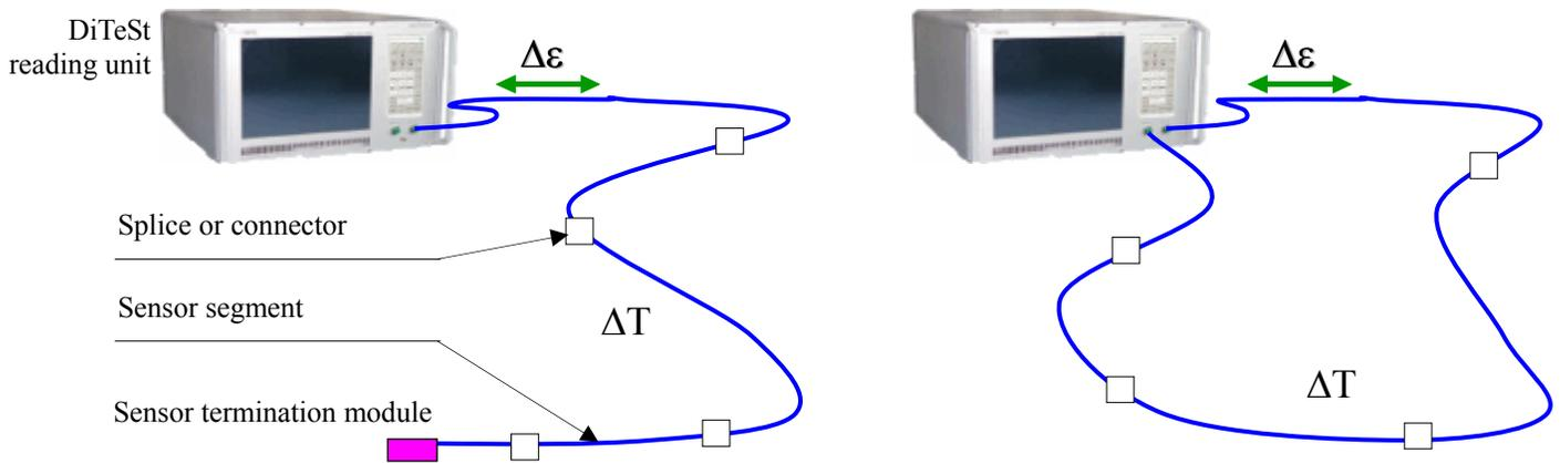
**Fig. 1: Schema of DiTeSt® system configurations, left: single-end configuration; right: loop configuration**
