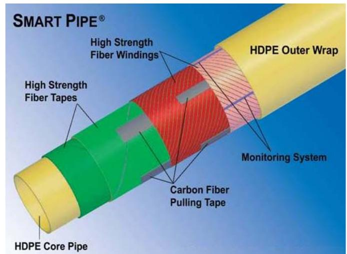
Figure 13. SmartPipe design, including SMARTprofile Monitoring system.
