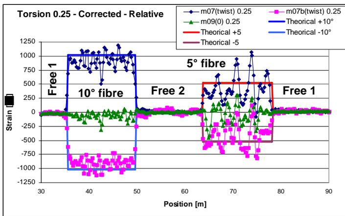
Figure 17. Results of the torsion test and comparison with theoretical predictions; higher winding angles provide more sensitivity and accuracy for torsion measurements
