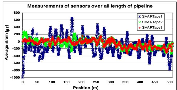
Figure 9. Strain distribution over the monitored part of the pipeline measured by SMARTape sensors
