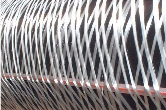
**Figure 14. SMARTprofile integration with high-strength fiber windings.**
