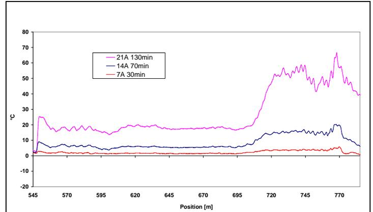
Figure 19. Liner temperature changes for different current levels and heating times. The first 545 m of optical fiber are not integrated in the liner and not shown
