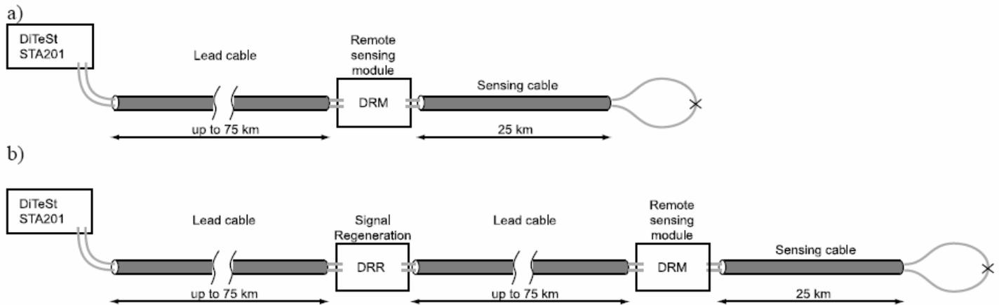
**Fig. 2: Range Extender Configurations, allowing the monitoring of long pipeline sections with a single instrument**
